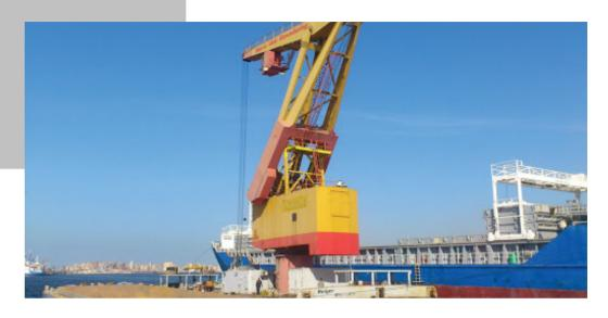
Grains & Feed Materials Transshipment Operations (floating ship-unloader at Alexandria port inner anchorage, Discharging Capacity 600 Tons /Hour.
